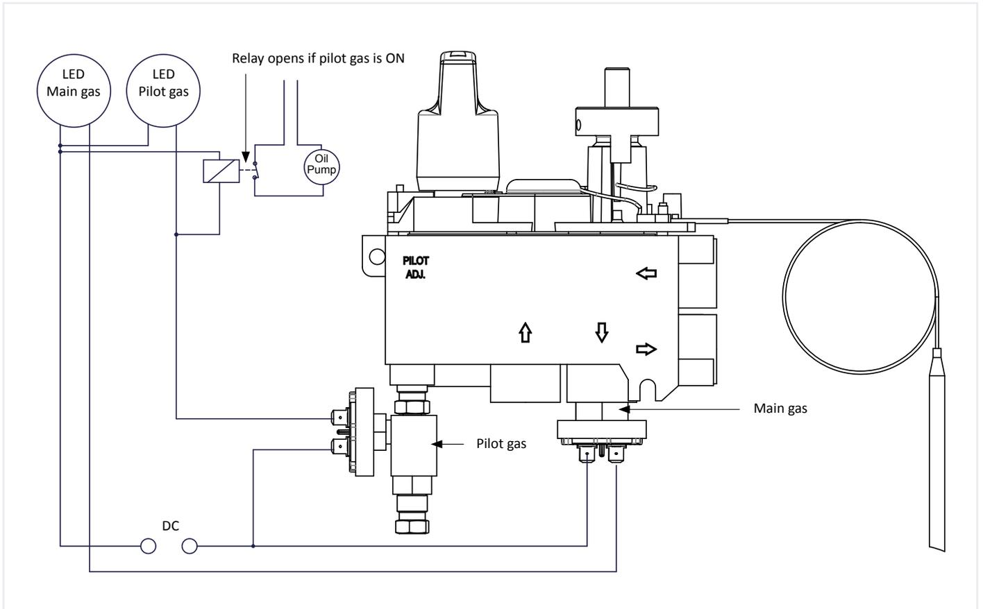
Fig. 5: Pilot gas and main gas installation
