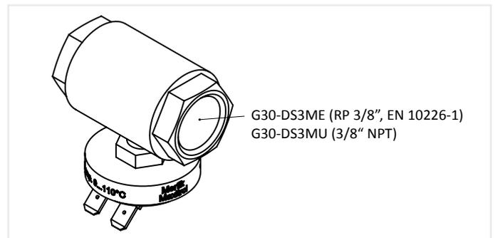
Fig. 2: Switch with adapter to pipe – Main Gas
