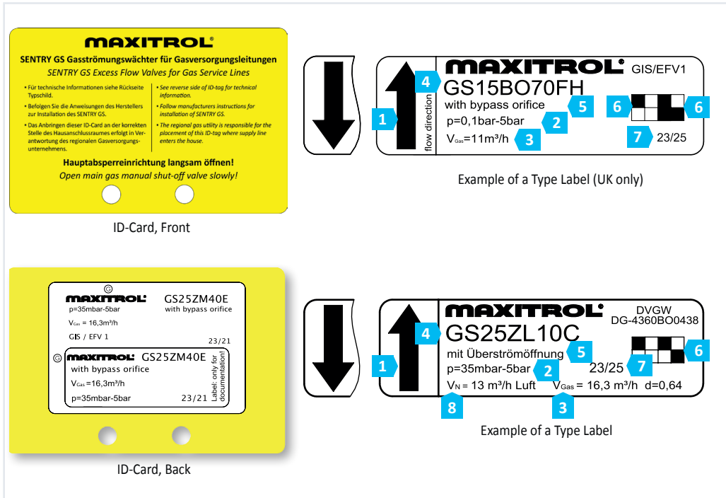
◀ Figure 7 SENTRY GS ID-Card (with type label on the back) for mounting on the main gas shut-off valve; Example of a type label
