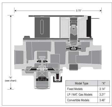
**Note:** Dimensions are maximums and are to be used only as an aid in designing clearance for the regulator. Actual production dimensions may vary somewhat from those shown. All other dimensions are as cast  $\pm$  0.05 inch. Maxitrol Company reserves the right to change specifications without notice.
