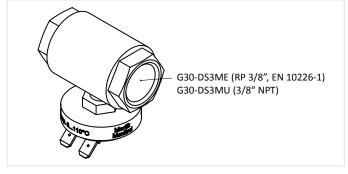
Fig. 2: Switch with adapter to pipe – Main Gas
